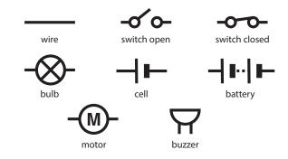
When getting the children to draw circuits, these should be completed with a ruler to make square circuits, rather than free-flowing wires. The positive end of the cell (single battery) is the longer line. A series of single batteries (cells) makes a 'battery'.
