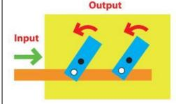
When you push the card strip (input movement), the two levers move (output movement).
